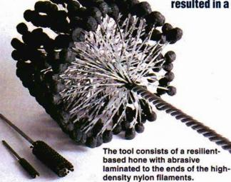
Haskel Inc. (Burbank, CA) manufactures a variety of compressed air driven pumps for use in a cross-section of industrial applications. The company experienced quality control issues with the manufacture of its miniaturized models. Burrs are created in the air drive system's aluminum sleeve, which must meet specification of 16 micro-finish.
