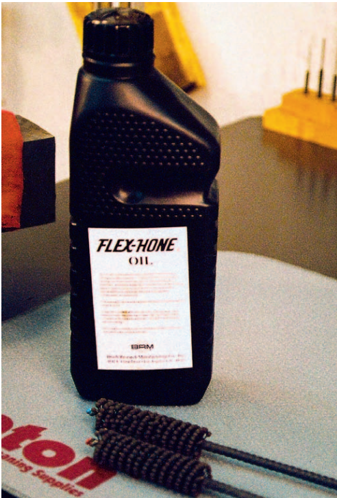
The Flex-Hone, which is composed of hundreds of small abrasive balls mounted on individual nylon bristles, and Flex-Hone Oil allow you to polish a shotgun's bore easily with an electric drill.
