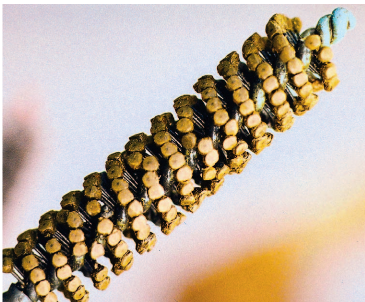
As the Flex-Hone is turned in the bore, the individual abrasive balls wear down.
