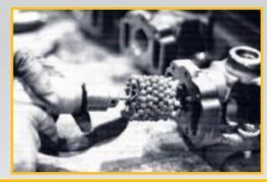
Operator can eliminate the burr around the cylinder's port in two seconds. Hone features 180 grit silicone carbide abrasive on high-density filaments.
