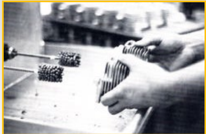
During the honing operation the operator deburrs each cylinder with several strokes, then switches the cylinder in his hands and repeats the process.
