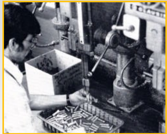
Operator begins final deburring operation on the inside diameter of the aluminum sleeve used in M-series compressed Air-driven pumps Manufactured at Haskel Inc.'s Burbank, CA facility.
