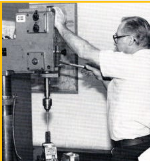
Operator prepares to deburr part for a hydraulic tool at the ENERPAC Butler Wisconsin facility.
