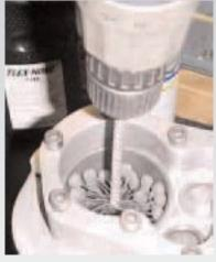
reason we recommend differing final grit sizes is our experience with the resulting ring seal. Prior to using the Flex-Hones for your final finish, the cylinder should be cleaned of the honing slurry left from the positive pressure hone. A clean rag with carburetor cleaner or WD40 will do a good job at this stage.
