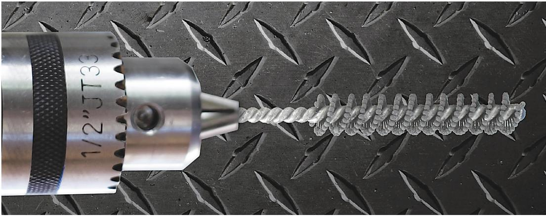
In combination with Heule cutting tools, a major jet engine component manufacturer applies the Flex-Hone from Brush Research Manufacturing on the machining center for final deburring of through-holes, which is usually an expensive and time-consuming manual operation.
