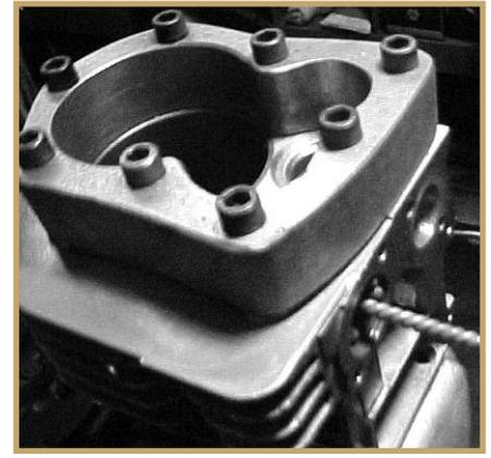
Assumption: They had used a Micromatic type automatic with a diamond stone. Perhaps the stone was worn unevenly because of the ports and may have “bounced” causing out-of-round, and the stones may have become tapered causing almost no cross hatch or finish at the plug end of the cylinder, where it is needed most.
