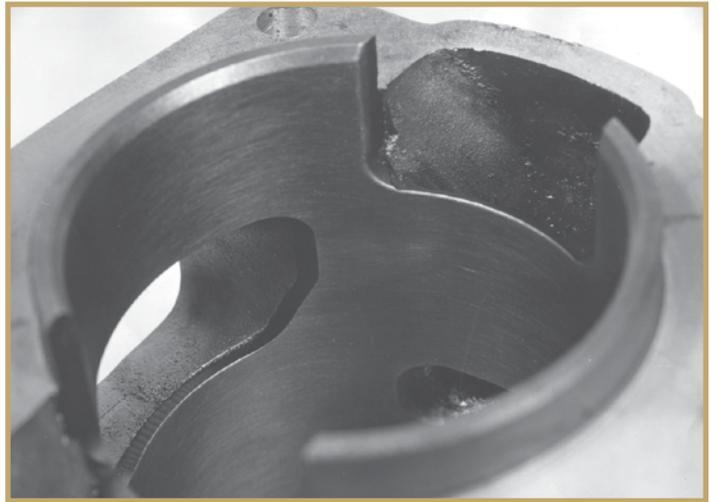
One U.S. Company who makes small ported engines has constructed a machine to take a group of barrels at a time. The Flex-Hone is rotated and actuated 15 seconds to the left, then 15 seconds to the right. The ports are deburred, and the proper cross hatch is put into their flash-chromed cylinders. Not only do they save a lot of time (money in manufacturing), but they report fast ring seating, and much better performance and longer engine life.
