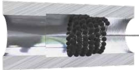
Although large-diameter flexible ball-style hones are somewhat unique, they are needed to resurface liners and cylinder bores in larger engines such as the Worthington, Clark, Ingersoll-Rand and Cooper-Bessemer models used for heavy-duty applications.
