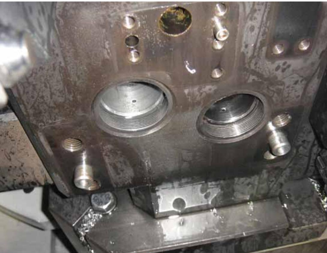
**The cavity on the left has been finished with the Flex-Hone tool. Finishing with the ball-style hone in the field gives cylinder cavities a super high finish that is virtually unattainable through the use of standard cutting tools, according to Brush Research Mfg. Co.**
