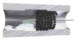
Although large-diameter flexible ball-style hones are somewhat unique, they are needed to resurface liners and cylinder bores in larger engines such as the Worthington, Clark, Ingersoll-Rand and Cooper-Bessemer models used for heavy-duty applications.
