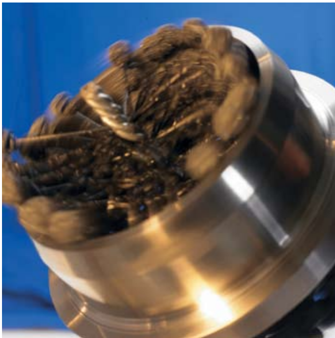
Flexible ball-style hones are available in various grit sizes and diameter sizes.
