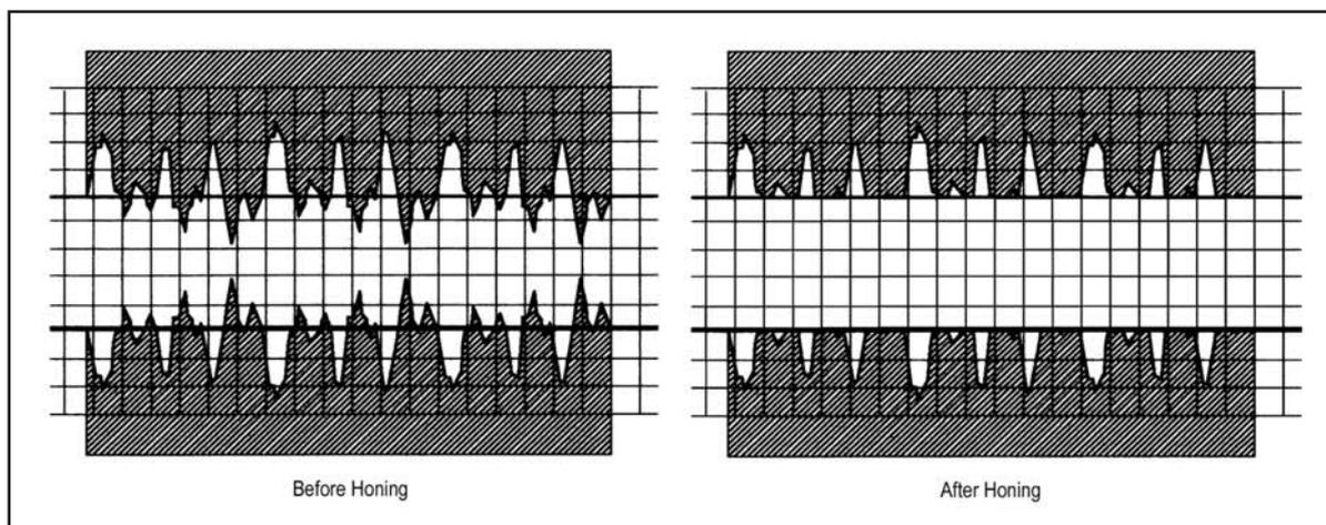
*Build up of wax or other solids may prevent proper valve operations or block lubricants. Proper maintenance tools, like the Flex Hone from Brush Research Manufacturing, leave a super-smooth plateau finish*
