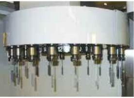
"Depending on the die, we use multiple hone sizes as well as varying grit materials and number of strokes," Taylor says. He adds the surface finish of the RCBS steel dies is sub-micron (roughness value) when they come off the machine. After the Flex-Hone finishing operation, the surface finish is improved by a factor of eight.
