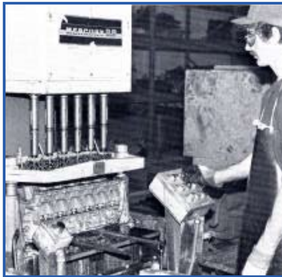
Operator pushes a button to start machine. Hones oscillate inside cylinders and expand as they exit, removing burrs created at port area during boring.
